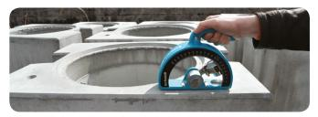
**Type PT:** Equipped with a larger plunger surface, it is especially designed to test on softer material such as light weight concrete, gypsum boards and on fresh concrete. It is often used to determine the right time to remove formwork.
